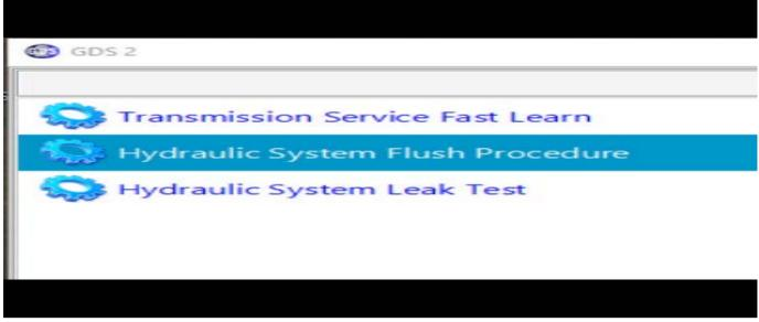
9. Select the Hydraulic System Flush Procedure.
