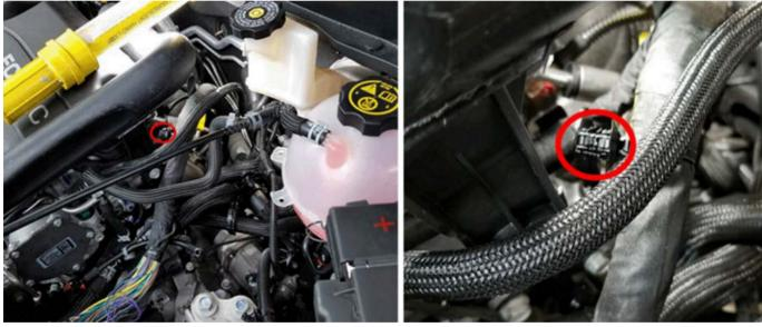
· Wire harness retainer not installed into bracket.
