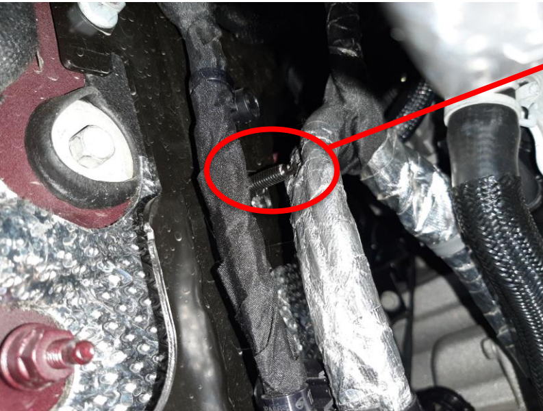
Hole Is Harness Thermal Sleeving From Stud
