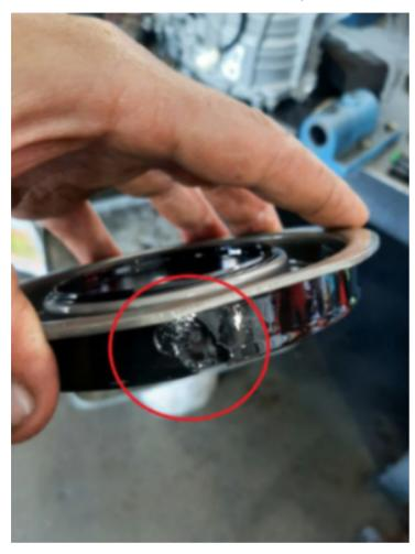
If the Forward clutches are worn and there is damage seen to the Forward Clutch Piston then replace the Foward Clutch Piston and Housing and the applicable apply components as needed
