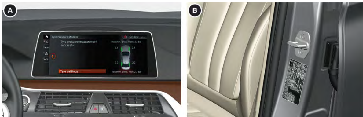
Electronic tire pressure specification in the CID of a G30 and tire pressure specification sticker on the B-pillar
