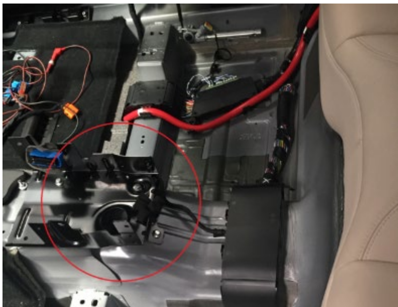
Figure 2: Harness containing the I-CAN line (white wire and blue wire) for the HVACR control unit (complete tunnel cabinet and rear passenger compartment carpet have been removed).
