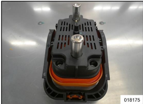
Figure 25: Manual service disconnect
