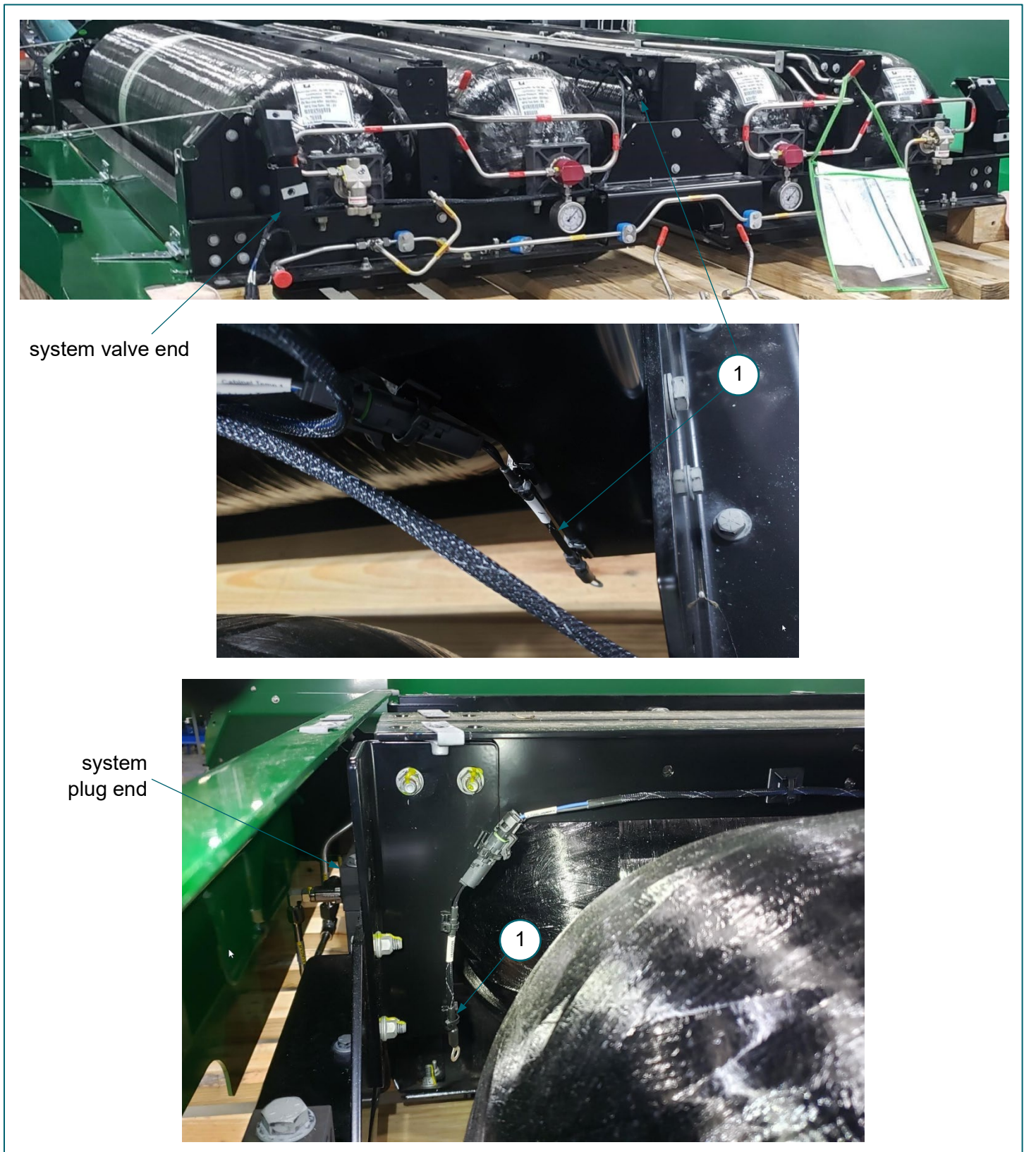
FIGURE 19b. Gen 3 Refuse Roof Mount (RM) Thermistor Locations
