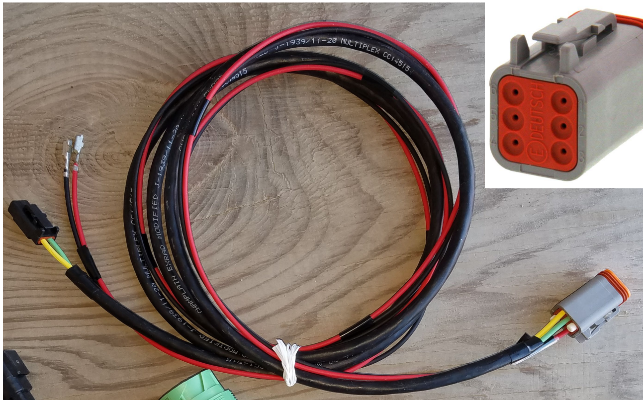
FIGURE 2-6. Blue iQ gauge harness and wire connector end view ( inset ). NOTE: Partial harness circuit shown; Blue iQ gauge harness connects to SAE J1939 circuit harness; refer to Section 2.10.
