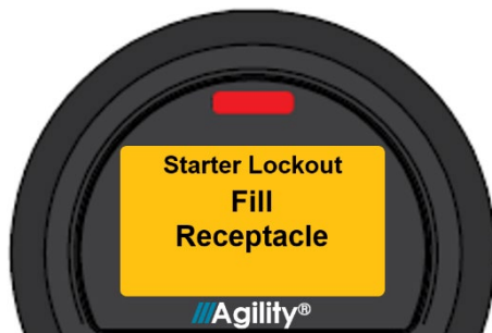
FIGURE 2–24. “Starter Lockout—Fill Receptacle” Blue iQ gauge warning message
