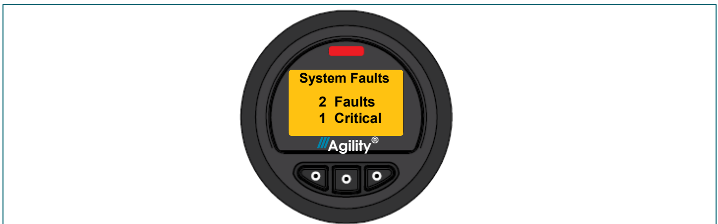
FIGURE 2–3. Blue iQ gauge screen indicating multiple system faults
