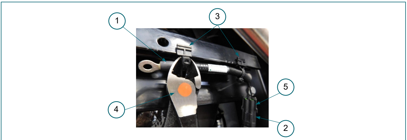
FIGURE 2–22. Use side cutters to remove edge clip zip ties from thermistor assembly
