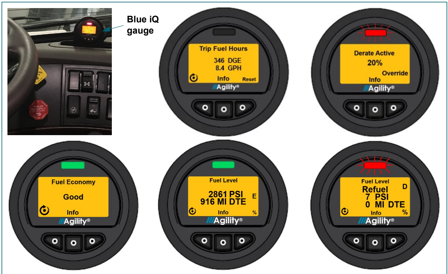
FIGURE 2–2. Blue iQ gauge and sample Blue iQ gauge screens
