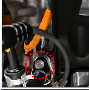
12. Remove the hose from the PCV Check Valve and reuse the soft line during reassembly.
