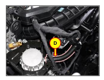
Remove the hose clamp that secures the soft line from the PCV Check Valve to the hard line under the Intake Manifold. Disconnect the soft line from the hard line.
