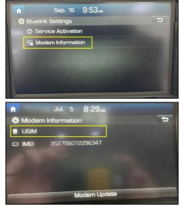
5. If USIM information is missing, capture photo using STUI in the GDS and proceed to **Section B**.
