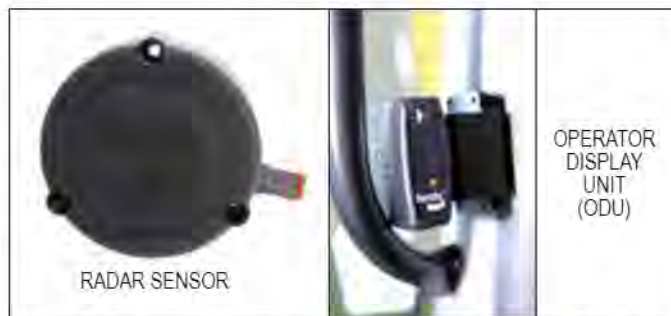
FIGURE 1 - BENDIX™ BLINDSPOTTER® RADAR SENSOR AND IN-CAB OPERATOR DISPLAY UNIT (ODU)
