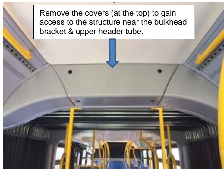
FIGURE 1: SHOWN INTERIOR COVERS TO BE REMOVED TO GAIN ACCESS
