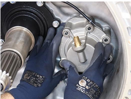
4. Ensure the Inertia Brake Piston Pin and Return Spring remain in the Lower Countershaft.
