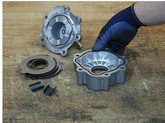
4. Install the 2 Wear Guides in the Inertia Brake Housing.
