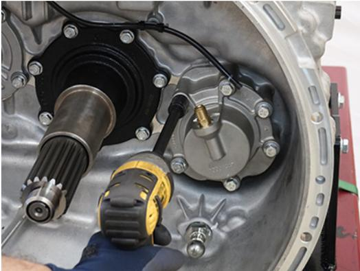
3. Remove the Inertia Brake Cover and Housing as an assembly. The original housing is not to be reused.
