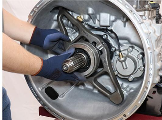
4. Push the upper end of the Release Yoke back until it locks to reset the LCA.
