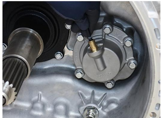
5. Install the Inertia Brake Cover onto the housing.
