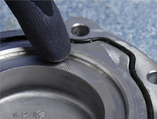
2. Install the new Upper Countershaft Cover O-ring (10001048) into the groove until fully seated.
