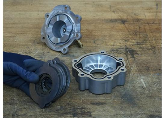
2. Remove the 2 wear guides from the Inertia Brake Housing.
