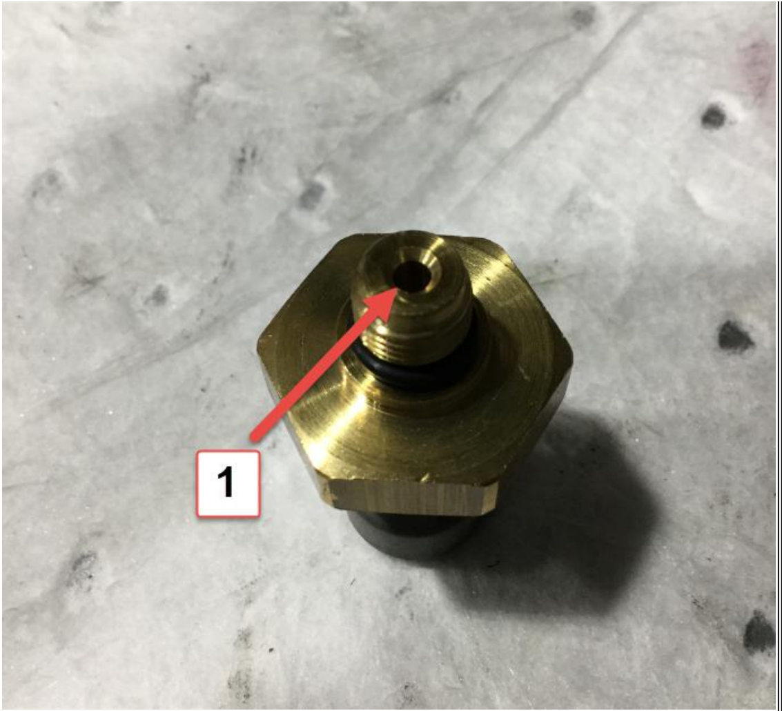
Figure 3: Intake Manifold Pressure (IMP) Sensor Item 1: Intake Manifold Pressure (IMP) Sensor Orifice
