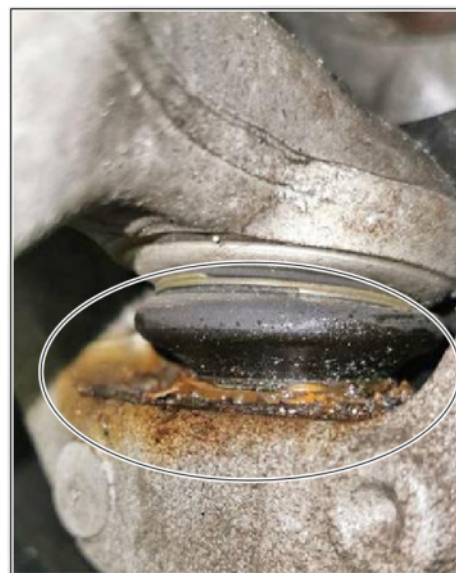
Example of grease leaks
