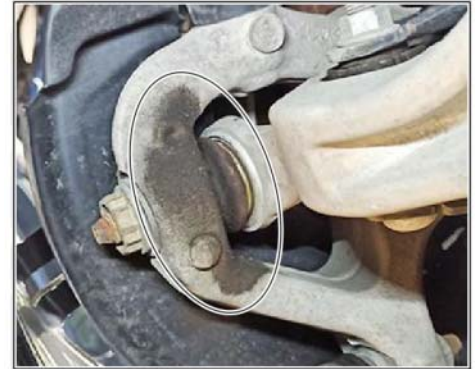
Example of grease leak 2
