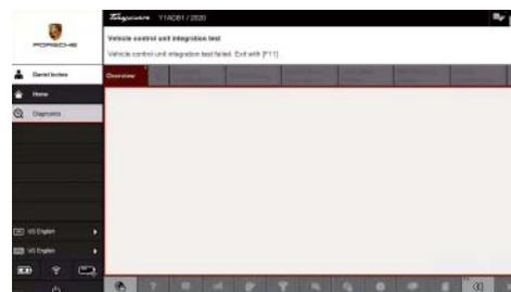
*Vehicle control unit integration test failed*
