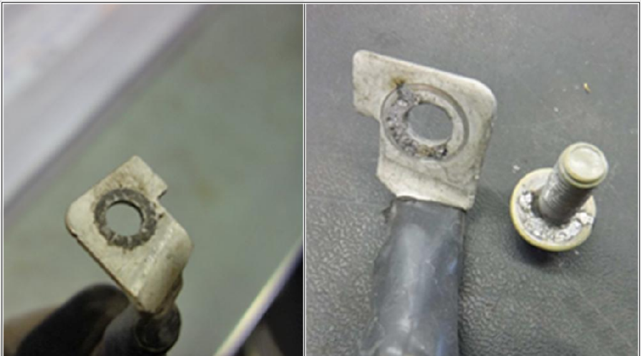
Fault type – ground strap and ground screws
