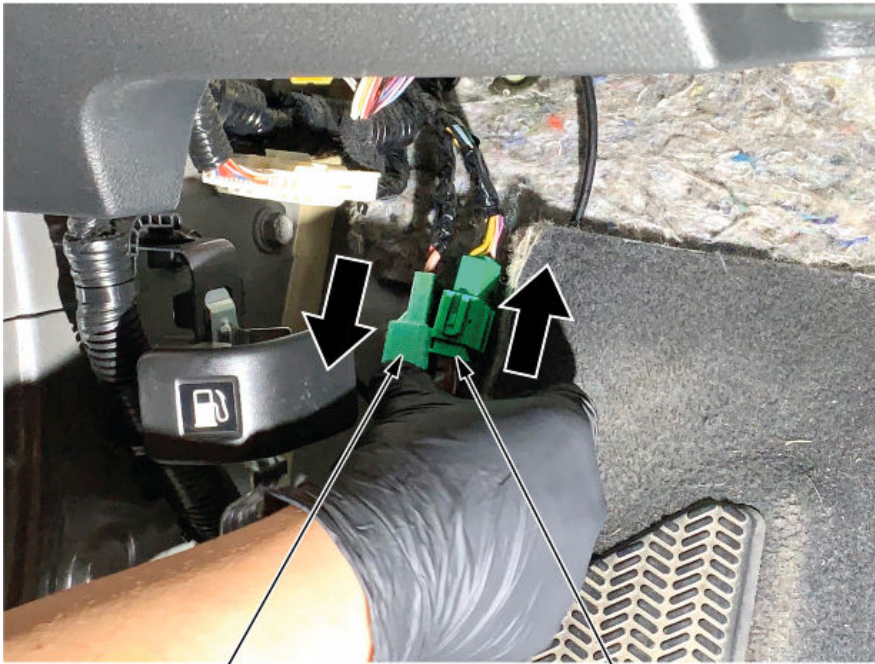
ENGINE ROOM HARNESS CONNECTOR Slide apart.
