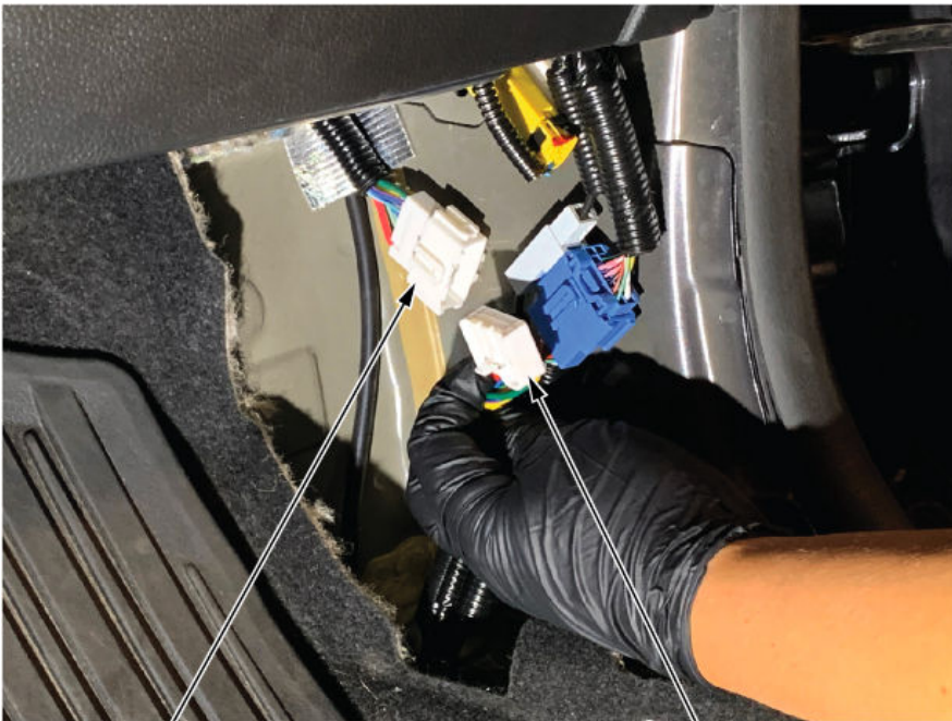
ENGINE ROOM HARNESS CONNECTOR Disconnect.
