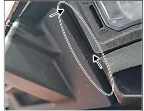
Gap between release and rear lid
