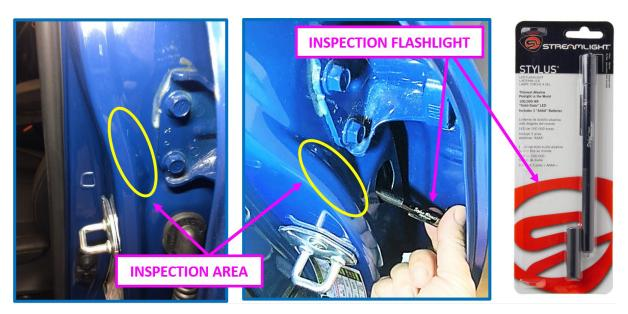
When practical, inspect the vehicle in a low light area or use your hand or a cloth to cover the area for easier observation of any light penetration. **NEVER** attempt to buff, grind, cut or polish this area prior to the inspection. Any actual splitting in this area will allow light to pass through with no additional prep required.
