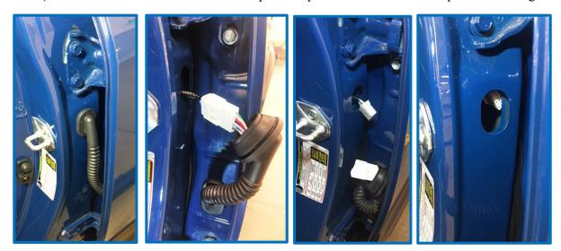
STEP 4) Shine the inspection light through door wiring harness hole. Be sure to aim the light in front of the upper left rear door hinge mount. A Streamlight® Stylus penlight was used in the example inspection photos below. Reduce the ambient light in the work area if needed. Examine the area closely for light shining through any splitting identified within the inspection area. See the **EXAMPLE** image of the splitting condition provided below.
