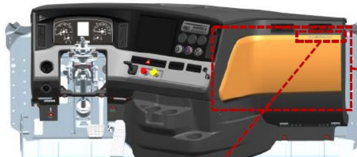
Fig.3, Electrical Bay Cover
