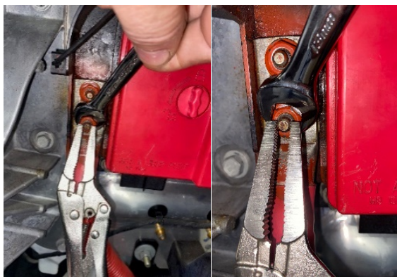
Fig. 5, Gripping the Stud to Tighten the Nut
