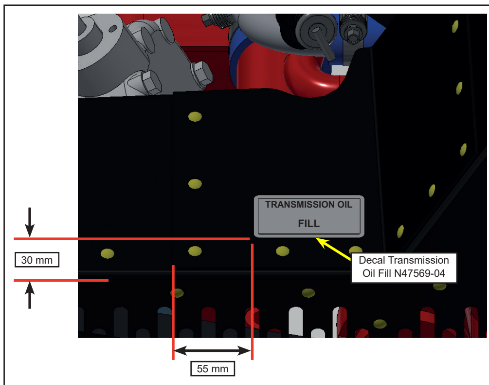
Figure 20 - Installation of Decal
