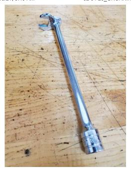
long extension, secure the lock nut at the back of the spindle.
