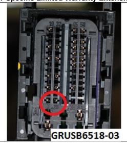
For the eligible vehicles with the **Electrical Machine Electronics (EME) wiring harness connector (A190\*1B), shown,** BMW of North America, LLC (BMW NA) is providing a repair-specific extended limited warranty to:
