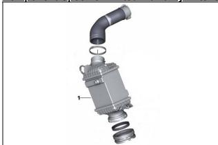
For the eligible vehicles, BMW of North America, LLC (BMW NA) is extending the limited warranty for the vehicle's **Charge Air Intercooler** to:
