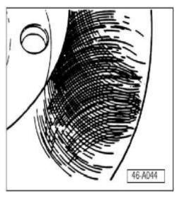
Replace sanding disc prior to moving to next Brake Disc surface.
