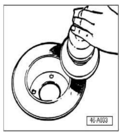
Remove remaining corrosion protection coating or surface rust as follows:
