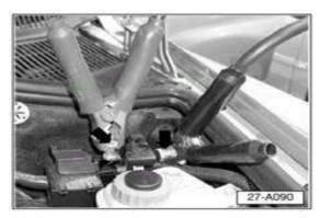
When using remote location terminals -arrows-, located in engine compartment, always reduce DIN rating on MCR340V, INC-940, VAS6161 and GRX3000VAS testers.
