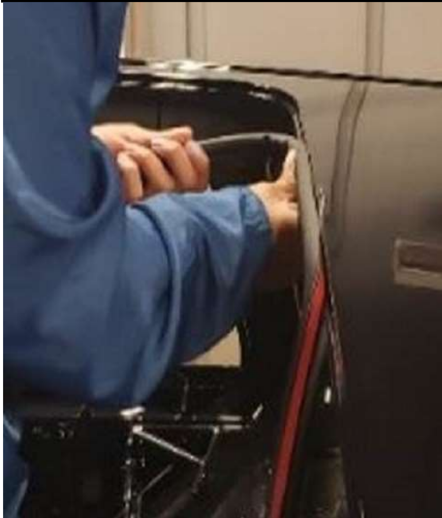
Figure 5: Example of installing the body side seal WITHOUT removing the “red” protective tape.
