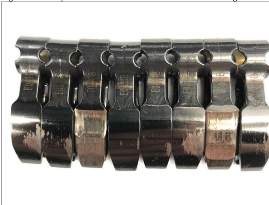
Figure 2: Examples of rocker arms with worn surface coating:
