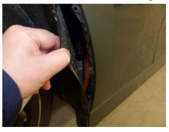
3. Clean the fender using R2 PN 83 19 0 417 324 around the area where the fender liner covers to prepare for inspection.
