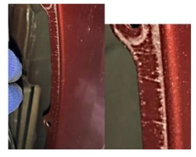
**Damage version 3:** Damage through the clear coat and paint down to the metal.
