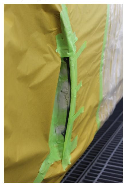
Step 14 – Pull the roll back tape back slightly 1-2 mm. Apply basecoat via SATA Mini Jet or similar with .08 fluid tip. Apply to primer areas first to achieve coverage, then blend out. Note in the picture the Spray gun is pointed inward away from the roll back tape edge to maintain a soft basecoat edge.
