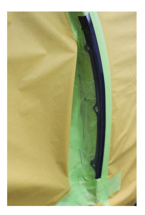
Step 9 – Mask the fender edge with a Roll Back tape – Masking tape should be minimum of 1 ½ inch width to provide a soft paint edge. Also prepare an open area at the top just above the upper rivet hole with a folded over 1 ½ piece of masking tape. The Folded tape will help provide a soft blend area at the top. Below are a few pics of the folded tape method.
