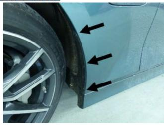
1. Remove the expanding rivets mounting the wheel arch cover to the front left side panel (rear area, three rivets) by punching through the locking pin, see image.
