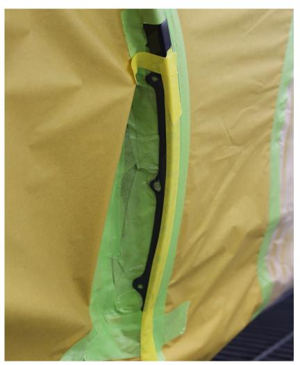
Step 8 – Remove the tape, clean, and prepare the area up to the outer fender edge with P- 2000 grit.
