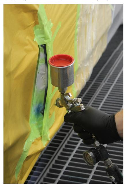
Step 15 – After basecoat flash off, pull the rollback tape back 1-2mm, as seen in the picture below.
