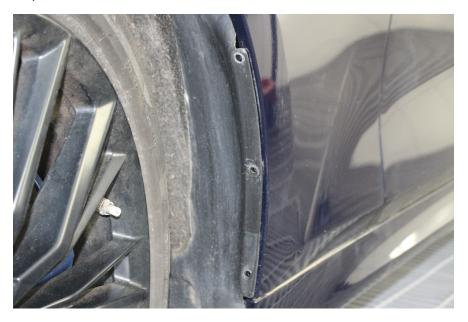
Step 3 – Pull back the wheel liner and tie off to wheel rim using a string or plastic tie.
