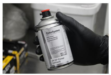
Step 11 – Properly mix the ColorSystem 2K EP Primer. Transfer the ColorSystem 2K EP Primer into a mixing container, recommend cutting a small notch in the lid to spray through and capture overspray. Approximately  $\frac{1}{2}$  ounce will be enough for two fender repairs.
