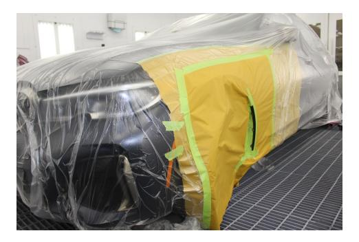
Step 7 – Clean and mask out damaged area just beyond the damage. Identified in the photo with yellow tape. This will prevent burn throughs when preparing the surface. Feather out the surface with P-500 - 600 grit to feather and remove corrosion. This will help prevent removing too much of the factory coatings.
