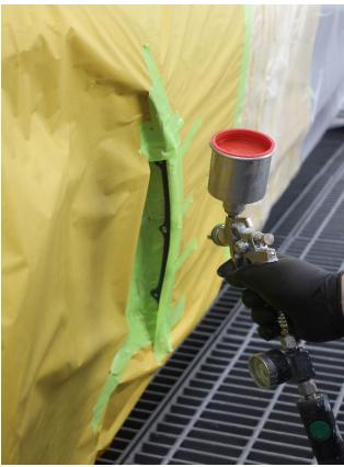
Step 13 – Set the SATA Mini Jet or similar @ 1 Bar (15 PSI) narrow the pattern to a bullet and in a controlled manner - apply two coats of 2K EP Primer to the bare metal areas. Each coat should be thin, and even to control overspray. While keeping a soft edge while achieving proper film build. Let flash for 20-30 min prior to applying basecoat.
