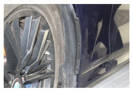
Step 2 – Remove the three rivets
