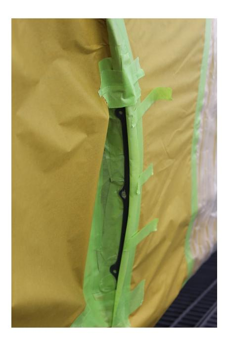
Step 10 – The bare metal must be coated with Epoxy Primer. ColorSystem 2K EP Primer Aerosol (51912347989). As the affected area is very small, a SATA Mini Jet or similar is the best method of application (.08 fluid tip).
