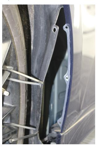
Step 4 – Once the liner is pulled back the area can be inspected for paint damage and corrosion. In this example there are a few areas with exposed metal and primer. Clean the area with Wax and Grease / Silicone Remover. (Market specific due to VOC compliance)
