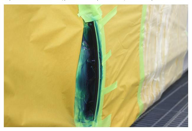
Step 16 – Apply Clearcoat with SATA Mini Jet or similar with .08 fluid tip. As with the basecoat and primer with the spray gun pointed inward to keep the edge soft near the rollback tape. If applying two coats of clear, pull the rollback away another 1-2mm before final coat. Directly after clearcoat application, remove the rollback tape and folded  $1\frac{1}{2}$  tape. Bake according to Clearcoat Technical Data Sheet.
