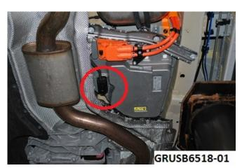
4. Perform a visual inspection of connector A190\*1B on the bottom of the EME.
