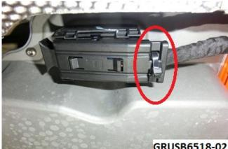
5. Remove connector A190\*1B from the EME. Cut the cable tie holding the harness to the EME connector.
