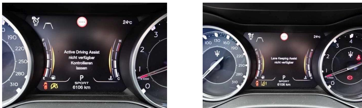
Figure 1: Warning messages related to ADAS functions unavailability. On the left “Active Driving Assist | not available | Service required”, on the right “Lane Keeping Assist | not available”.
