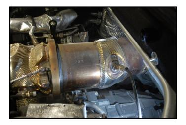
Inspect catalyst part numbers and replace, if necessary.
