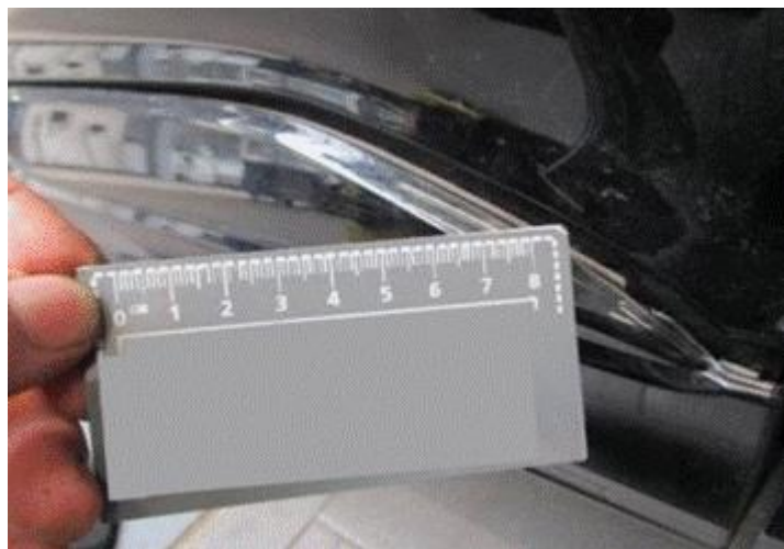
Figure 1. Debonded door trim cover and extent of detachment.
