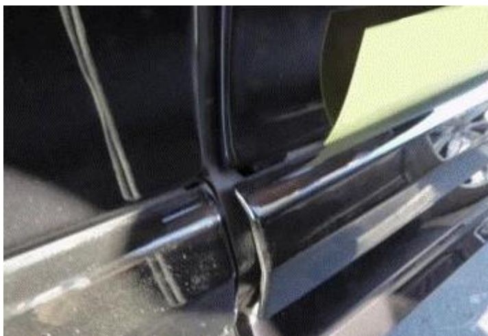
Figure 2. Alternative view of debonded door trim cover.
