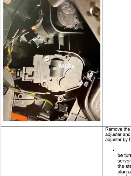
Remove the servomotor of the mixed air flap adjuster and attempt to turn the mixed air flap adjuster by hand.
