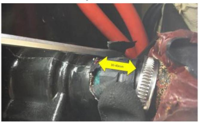
Install the new filler pipe as shown following the repair instruction. **NOTE:** <u>Do not</u> install the insulating tape that is described in the repair instructions.
