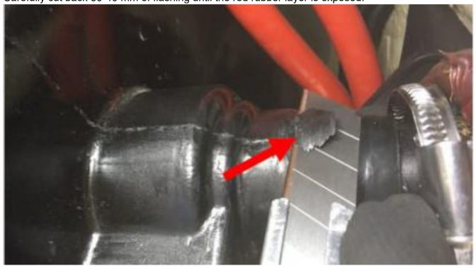
Remove that cut portion of black layer to expose the filler pipe.
