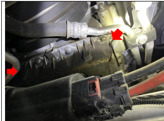
Example: B N63T Upper Oil Pan Gasket
