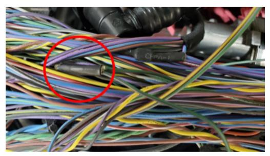
Inspect each leg for broken wire strands and correct any issues. Slide the appropriate size heat shrink tube up one branch of the circuit. Install a new splice clip, solder the three legs, and cover with the heat shrink. Close the main engine wiring harness using the appropriate PET under hood tape.
