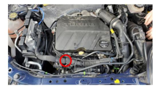
A high resistance splice in the main engine wiring harness above the EVAP Purge Pump, may cause the P0521 to set.
