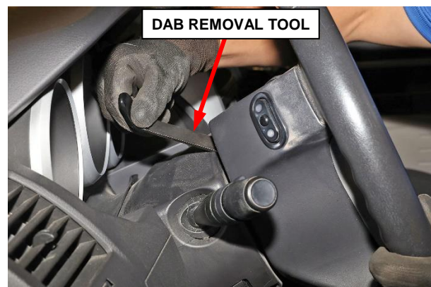
Figure 2 – DAB Removal Tool
