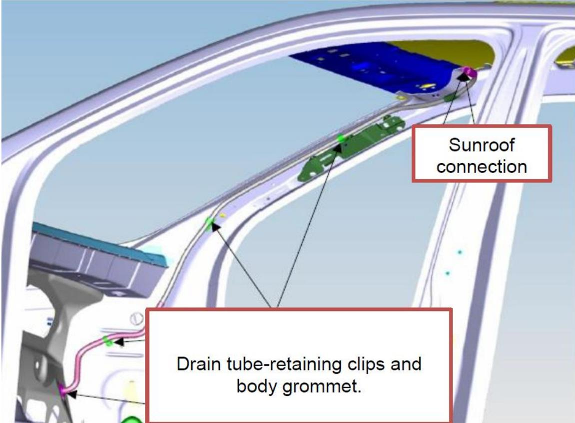
Sunroof front passenger drain tube routing
