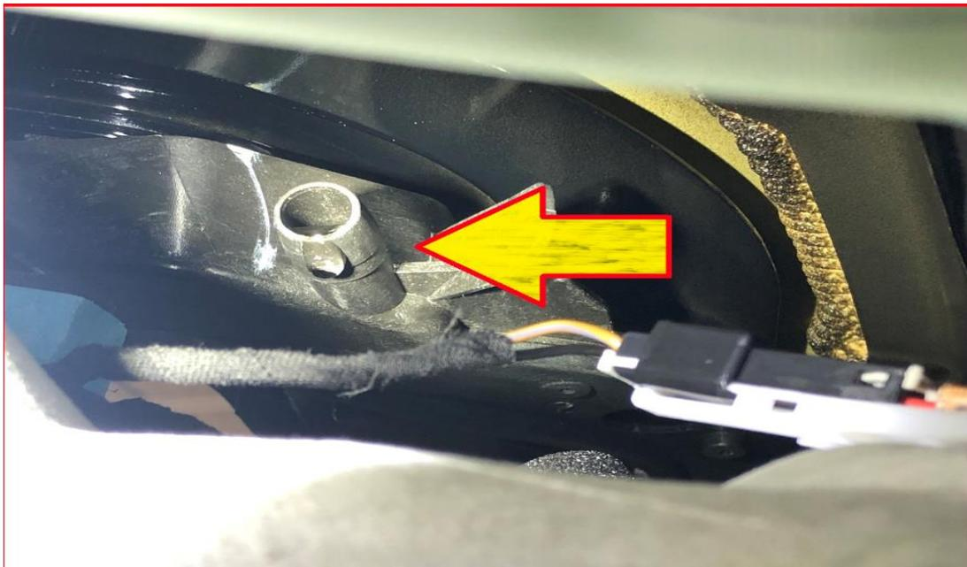
Missing Sunroof front passenger drain tube
