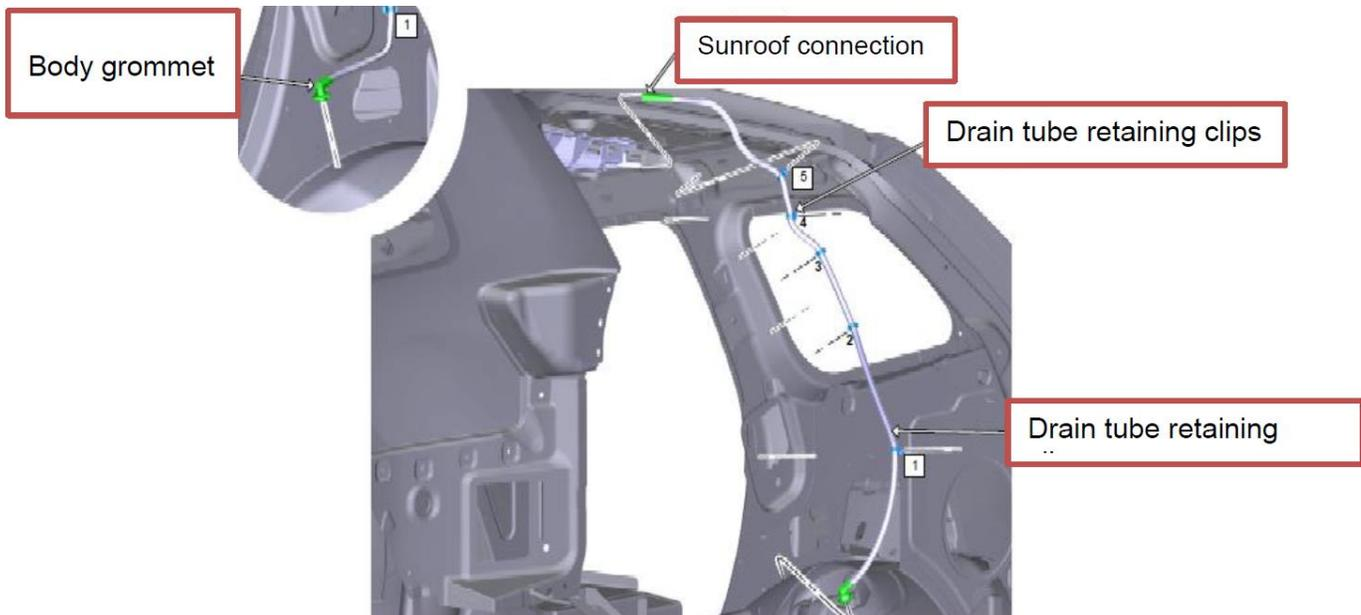
Sunroof, rear drain tube routing, passenger
