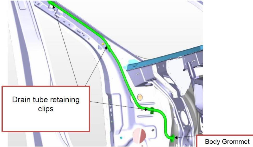
Sunroof, front driver drain tube routing
