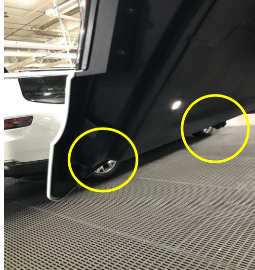
Fig 1 Gate Bumper Location
