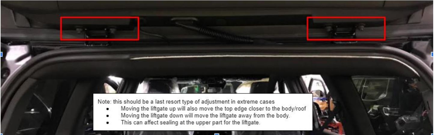
Fig 4 Gate Up/Down Fore/Aft Adjustment
