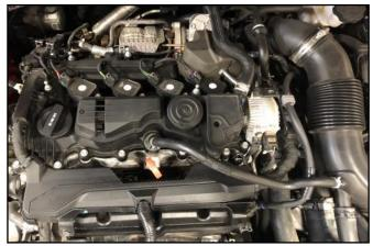
Complete a leakdown test on the affected cylinder exhibiting a misfire. If leakdown is 15% or greater, locate the source of escaping air.
