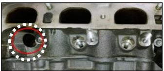
Upon removal of the GDI Injector, if injector has the appearance as seen to the right, replace the whole injector. Do not just replace the tip seal of the injector in this case.
