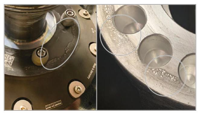
Material transfer on brake disc/wheel hub
