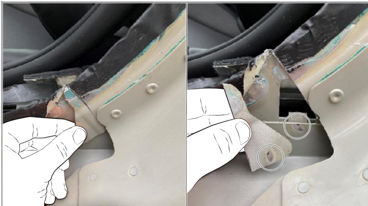
Example of sheet metal contact on unpainted bodyshell.
