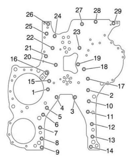
• Timing gear plate, tighten in sequence shown.....28 ± 4 Nm (21 ± 3 ft-lb)
