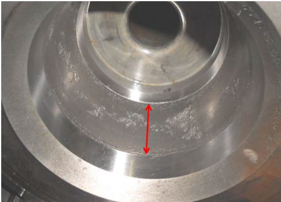
Spalled bearing race (Image 4)
