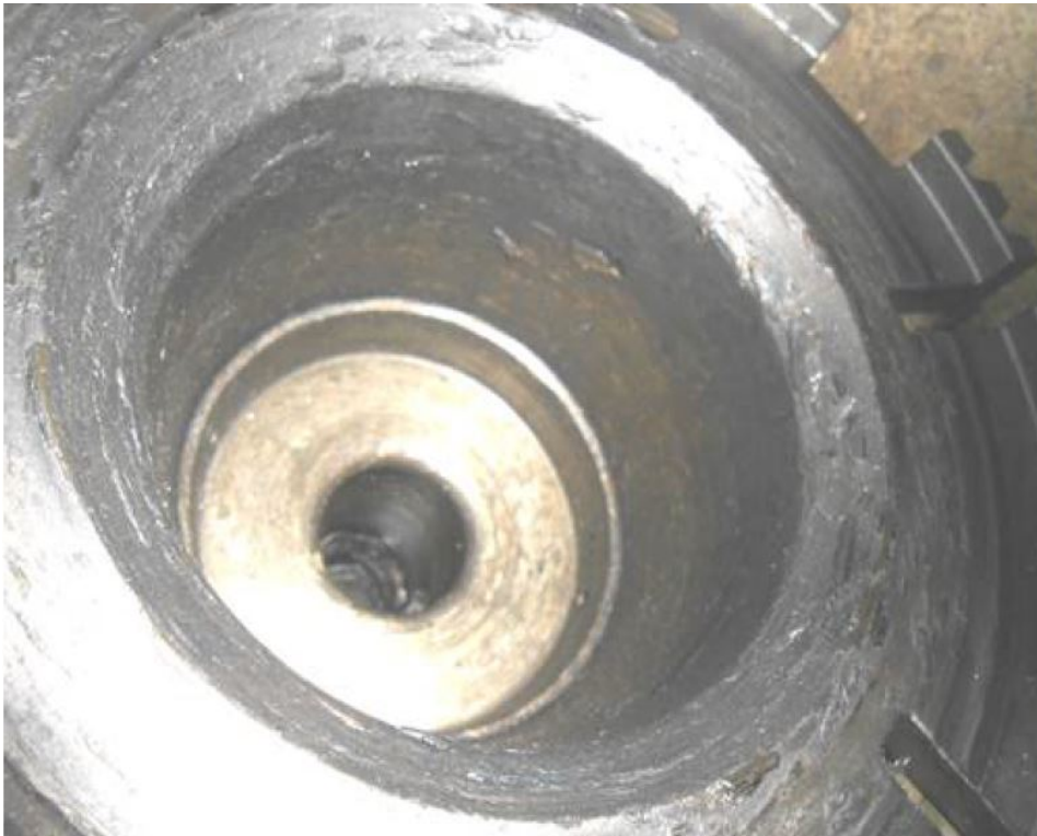
Spalled Bearing Race (Image 6)
