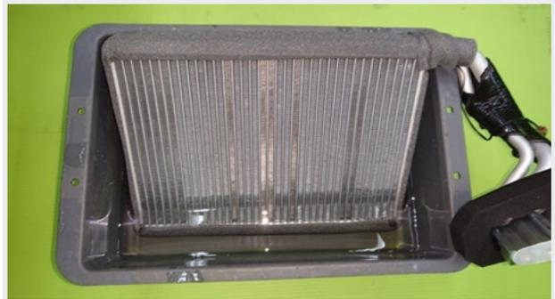
**STEP 3)** Remove the evaporator from the water after 5 minutes.
