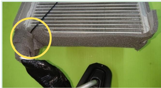
**IMPORTANT NOTE:** Make sure the lead wire is routed toward the end between the connector insulation and the evaporator insulation.
