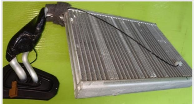
**STEP 4)** **CAREFULLY** remove the evaporator core insulation. Any remaining residue from the original adhesive is acceptable once it is completely dry.
