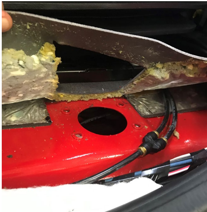
Fig. 20, Holes Drilled for Battery Load Disconnect Switch
