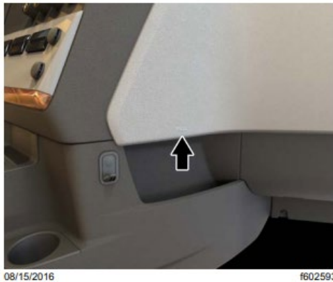
Fig.3, Electrical Bay Cover Handhold
