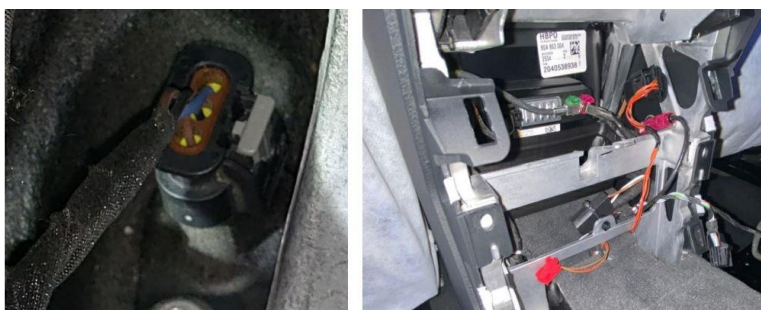
Figure 2. G28 crank sensor harness tight (left), Q5 Wireless charging pad harness tight (right).
