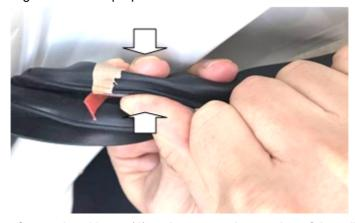
g. Peel off the yellow liner for another 10 mm (1) and press on that portion of the adhesive tape (2) to adhere to the seaming welt.
