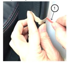
m. While holding the seaming welt so that it will not lift up, remove the red liner (1) by pulling on it.
