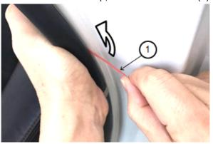
n. Press the seaming welt on with fingers where the adhesive tape is attached to ensure proper adhesion.
