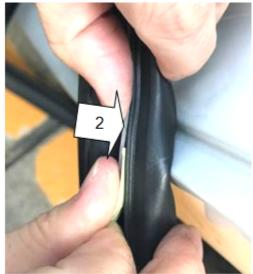
h. Repeat the previous step and attach the complete 250 mm of adhesive tape (1) to the seaming welt.
