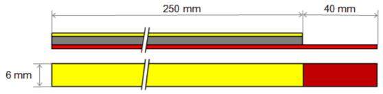
e. Peel off the yellow liner (from the side where the red liner is overlapping) for 30 mm (1) and attach the tape to the seaming welt (2), aligning the tape (3) edge with the dashed/dotted line.
