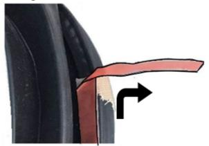
k. Clean the vehicle panel hemming part where the adhesive tape on the seaming welt will be attached.
